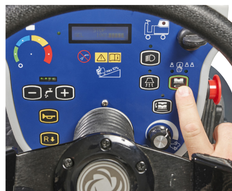
Brush deck/squeegee lowers automatically, minimising operator effort
