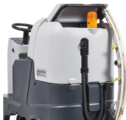
Squeegee hanger makes it easy to ride through closer spaces
