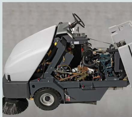
All major components are accessible quickly without the need for tools. Maintenance is fast and simple
