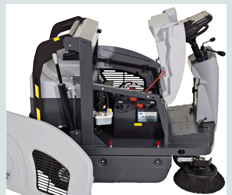
Maintenance is easy since no tools are needed for broom and filter removal and easy access to all components makes maintenance and service fast and easy
