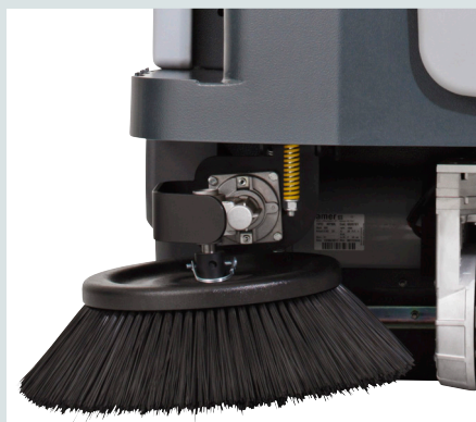
DustGuard™ misting system adds to the dust free sweeping improving the environment for operator as well as the surroundings (optional)
