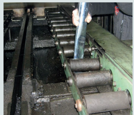
Vacuuming grinding sludge
